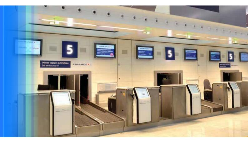
The Series 1 is an economical, easily deployable, retrofit model – integrated to the front of the existing check-in desk. The Series 1 Console is fitted with a hand-held scanner that enables passenger-operated bag tag scanning. The existing desks, conveyors and weigh scales are used, with the built-in ability to switch from self-service to agent-assisted modes of operation.
