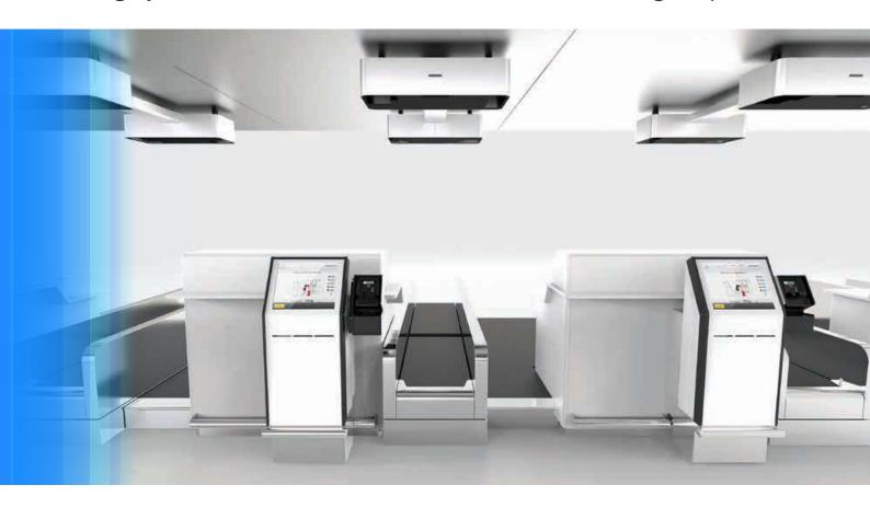
The Series 3 is a highly advanced automated bag drop solution, designed to be retro-fitted to existing airport infrastructure. A sophisticated sensor array is mounted above the conveyors that automatically reads the bag tag, and creates a virtual exclusion zone which prevents weight tampering and ensures passenger safety. No processing or movement of baggage will occur if there is an intrusion into the protected zone.
